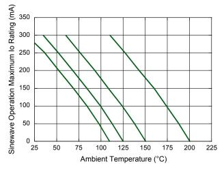
Sinewave Operation 50% Duty Cycle,  $R_{\rm BJA}$  (PCB) = 325°C/W. Maximum Finish-Alloy Temperature = 175°C
